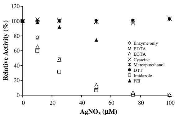
Fig. 4. Protection of creatine amidinohydrolase from silver-induced inactivation.
