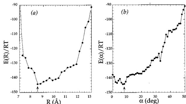
FIG. 9. Energies of the most probable configurations of a pair of idealized helices of  $n=30$  residues as a function of (a) the separation  $R$  between the centroids of the helices, and (b) the angle between the principal axes of the helices. The ordinate values represent the loci of the local minima located by the simplex algorithm for each fixed value of the geometric variable  $R$  in (a) or  $\alpha$  in (b). A global minimum is observed at  $R=8.5$  Å and  $\alpha=7.5^\circ$ .
